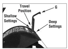
Figure 3-5: Depth regulator lever.
